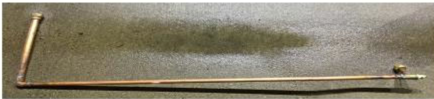
Figure 4: Removed Vacuum Assist copper Vapor Piping
