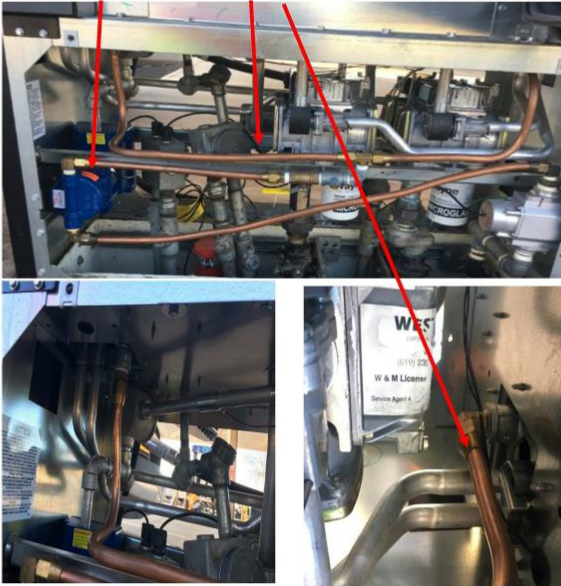
Figure 10: VP 1000 Vacuum Pump and Vacuum Assist copper tubing kit: Wayne Ovation.
