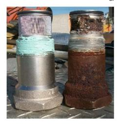
This photo shows swift check valves used with PLLDs on Red Jacket STP's.
