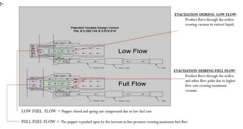
The net result is a lower pressure drop, with a corresponding flow rate increase: up to a 1 gpm higher flow rate over the competition.
