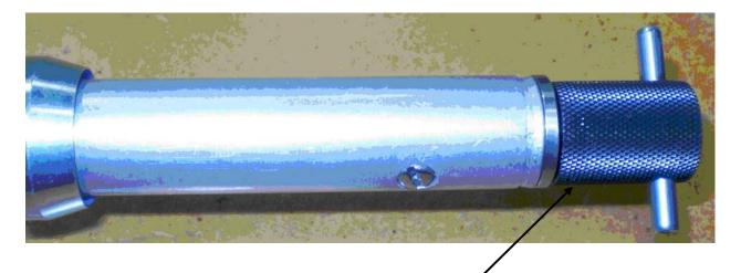
Plug properly inserted into nozzle spout. Both plug o-rings seated into nozzle spout.
