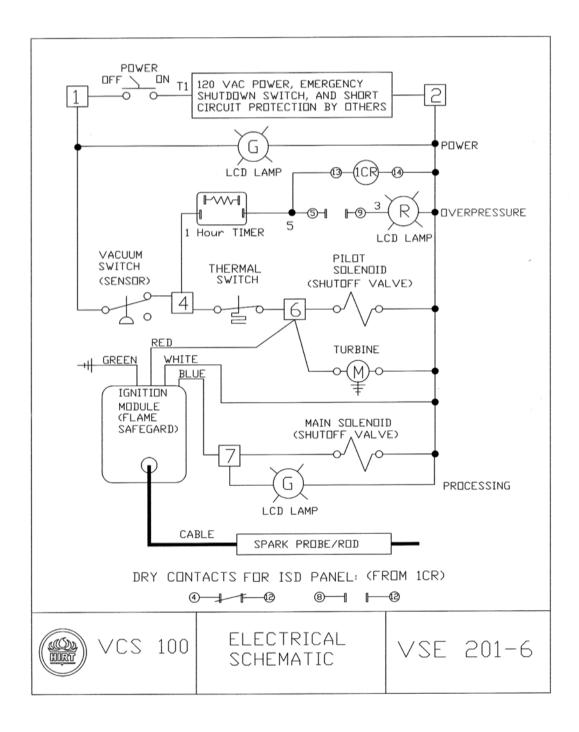
Note on the ELECTRICAL SCHEMATIC that a [1] to [6] jumper energizes the turbine, ignition module, and pilot solenoid. A [6] to [7] jumper energizes the main solenoid.
