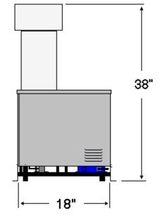
MODEL: VCS 100 SERVICE: Outdoor, non hazardous area ELECTRICAL: 120 VAC, 3 Ampere, intermittent VAPOR PIPE CONNECTION: 3/4@ NPT WEIGHT: 80 lbs. OVERALL DIMENSIONS: 18" wide X 18" deep x 38" high (without legs)
