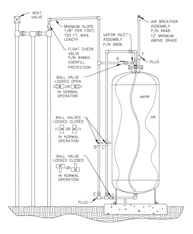
**Figure 1H**Normal Clean Air Separator Operating Configuration
