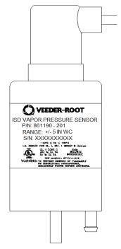
Veeder-Root Model # 861190-201 Low Powered Vapor Pressure Sensor
