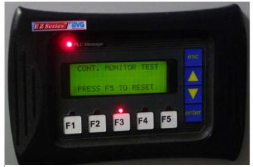
Figure 7: F3 Displays "Cont. Monitor Test"
