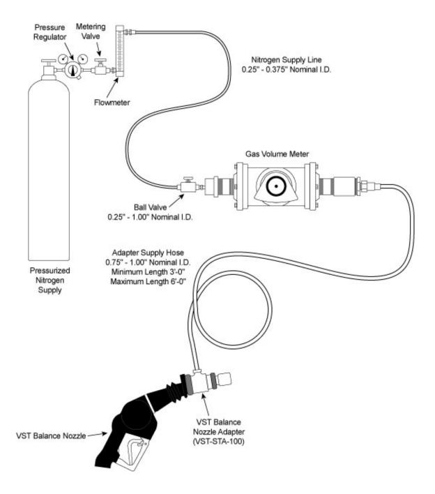
Figure 2.B Emco Wheaton Retail Vapor Flow Meter Test Assembly
