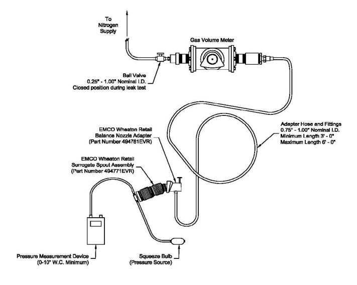
Figure 2.A VST Vapor Flow Meter Test Assembly
