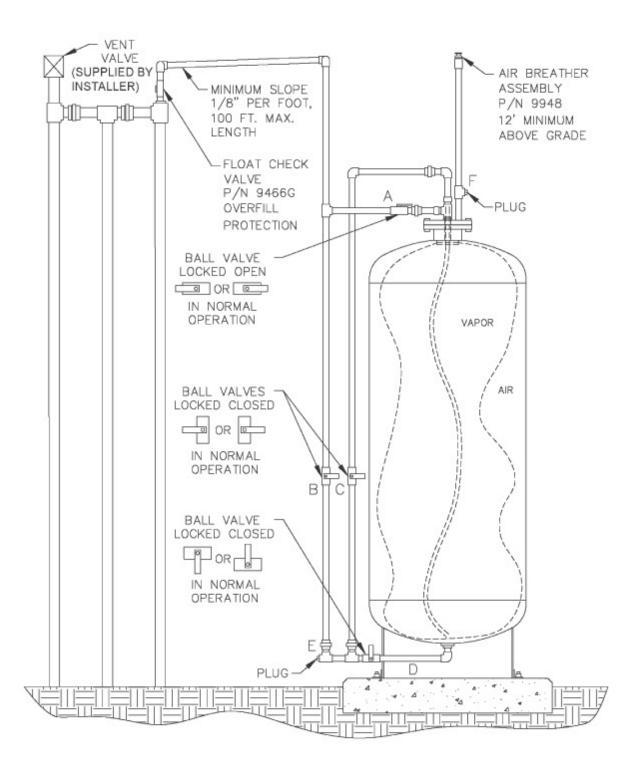
Figure 1A-11 Healy Model 9961 Clean Air Separator
