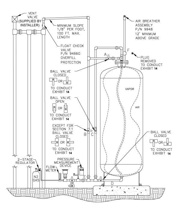
**Figure 2H**Clean Air Separator in Configuration to Conduct Test
