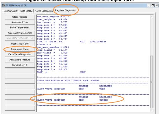
Figure 22: Veeder-Root Setup Tool-Close vapor Valve
