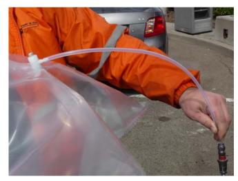
Figure 4: Attach Tedlar Bag to Vacuum Pump to Evacuate the Nitrogen
