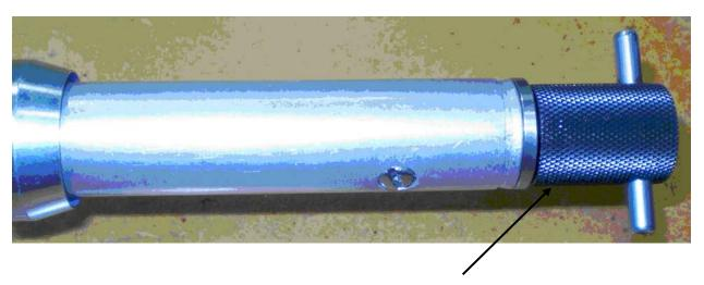
Plug properly inserted into nozzle spout. Both plug o-rings seated into nozzle spout.
