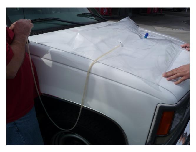
Figure 2: Tedlar Bag Connected to Nitrogen
