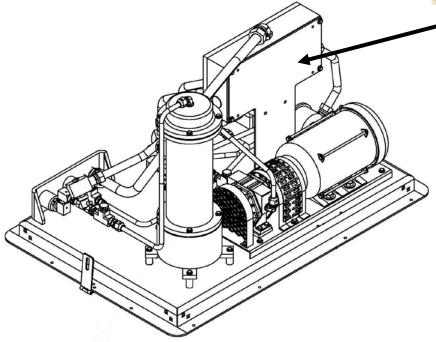
Label with serial number is located inside the Green Machine housing on the electrical junction box.
