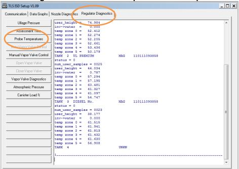
6.2.16. To switch the vapor valve from automatic to manual control or visa versa, select the "Regulator Diagnostics" tab at the top of the screen and select "Auto Vapor Valve Control" or "Manual Vapor Valve Control" to toggle between these two options. See Figure 19 and Figure 20. If "Manual Vapor Valve Control" is selected then "Open Vapor Valve" or "Close Vapor Valve" can be selected. See Figure 21 and Figure 22.
