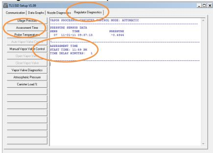
6.2.15. To access the probe temperatures, select the "Regulator Diagnostics" tab at the top of the screen and select "Probe Temperature" on the left side of the screen. See Figure 18.
