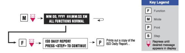
The ISD version number can be verified on the TLS Console LCD screen using the <STEP> key or by using the TLS Console <PRINT> key to print and review the latest ISD Daily Report:
