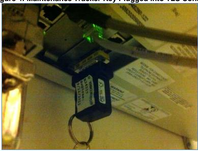
Figure 4: Maintenance Tracker Key Plugged Into TLS Console
