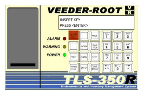
6.1.3. The Maintenance Tracker key (see Figure 3) must be plugged into a RS-232 port underneath the TLS Console within one minute or system will timeout. See Figure 4.
