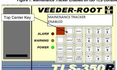
Figure 1: Maintenance Tracker Enabled on ISD TLS Console
