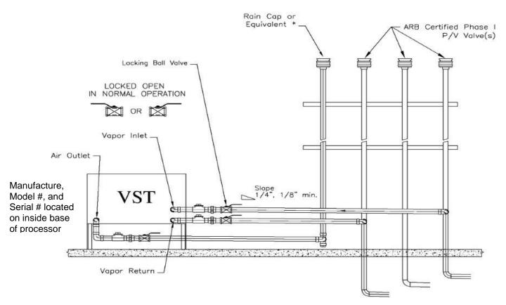
CAUTION: THE HANDLES ON THE LOCKING BALL VALVES MUST NOT BE REMOVED
