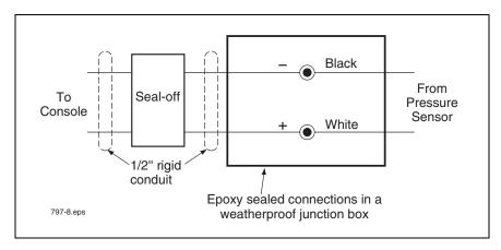
Figure 3. Field wiring Pressure Sensor - Observe Polarity
