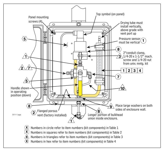
Figure 2. Mounting Pressure Sensor Assembly onto Composite Panel
