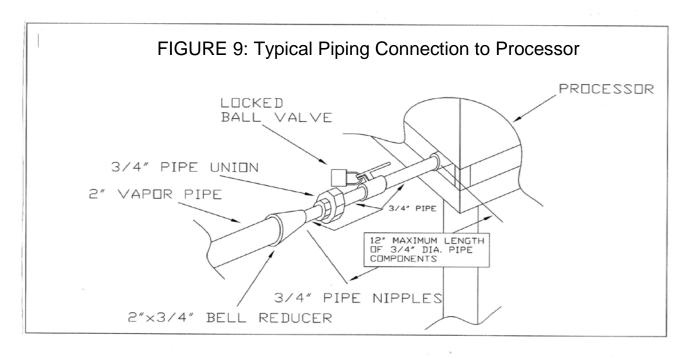
**CAUTION:** Hold processor internal pipe train with backing wrench to <u>prevent</u> twisting pipe train while connecting vapor piping.
