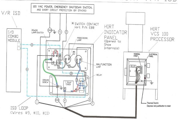
\*NOTE: ALTHOUGH SWITCH CONTACT IS SHOWN ON SIDE OF POWER LAMP/SWITCH FOR CLARITY, ACTUAL CONTACT MOUNTS (STACKS) ON BLUE COLORED SECTION OF SWITCH.
