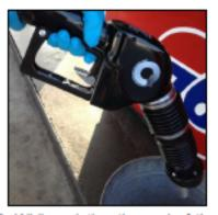
While pointing the end of the spout downwards into a gasoline approved container, engage (squeeze) the lever without compressing the bellows. Perform this step a minimum of three times to assure the lever has free motion and no tension (dead lever).
