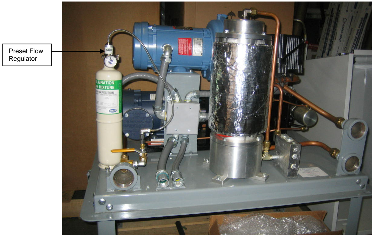
Figure 2 Equipment Configuration for Verifying Hydrocarbon Sensor Performance
