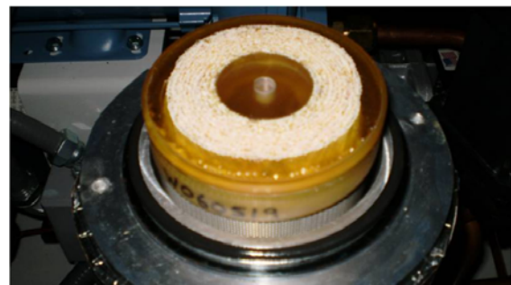
Figure 30: Exposed membrane with top plate removed.
