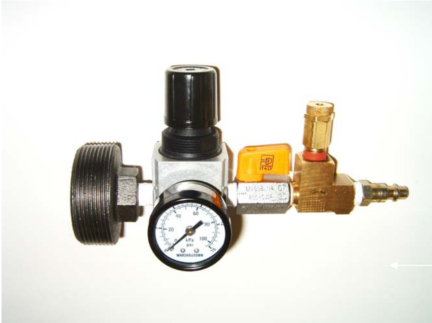
Figure 7: Typical Leak Check Test Fixture
