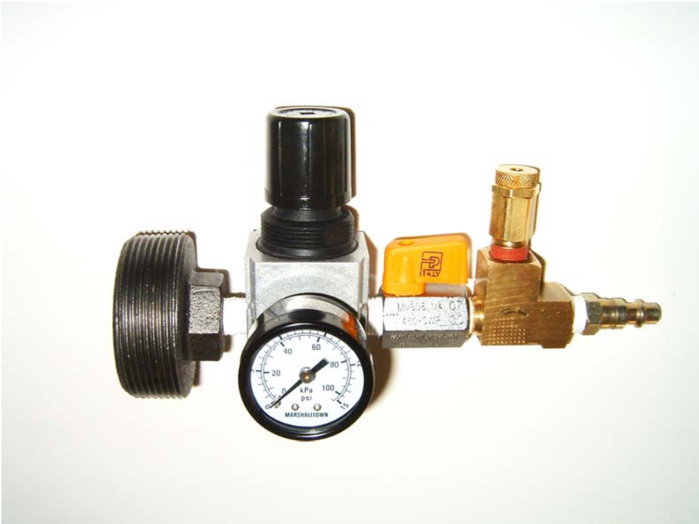
Figure 20: Typical Leak Check Test Fixture
