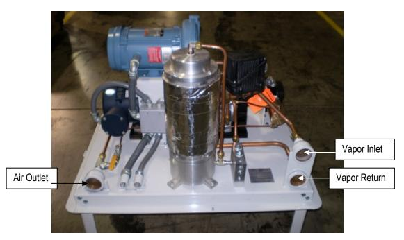
Figure 19: Processor Inlets & Outlets
