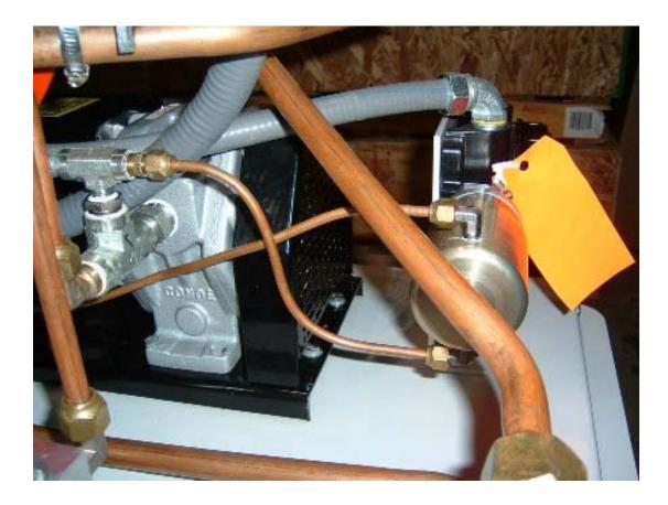
Figure 50: HC IR Sensor Module 1/4" 45° tubing and fittings
