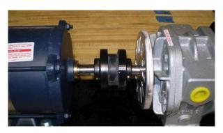
Figure 33: Vacuum pump with guard removed
