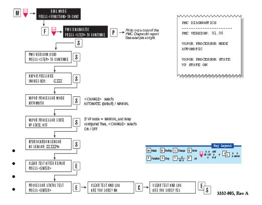
Figure 10: PMC Diagnostic Menu with PMC Software
