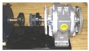
Figure 35: Vacuum pump unbolted and moved away from the motor
