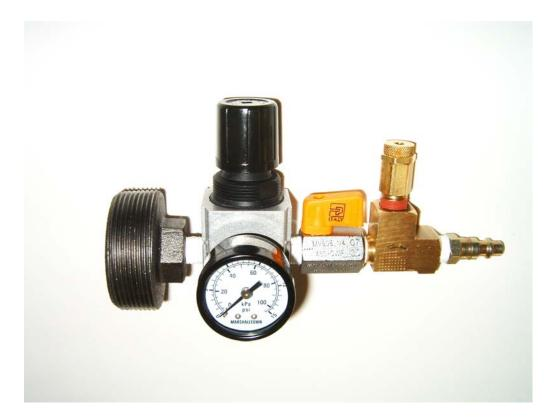
Figure 20: Typical Leak Check Test Fixture
