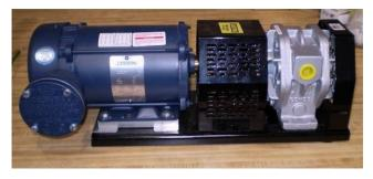
Figure 34: Vacuum and motor assembly
