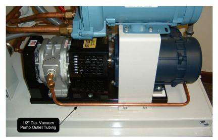
Figure 25: Vacuum pump outlet tubing connection
