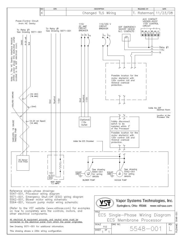
Figure 19: Processor Single-Phase Wiring Diagram
