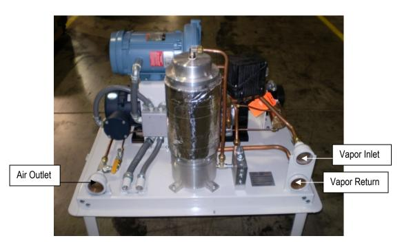
Figure 6: Processor Inlets & Outlets
