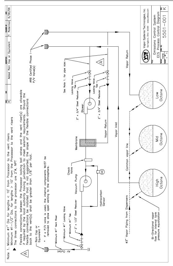
Figure 17: Processor Piping Connections
