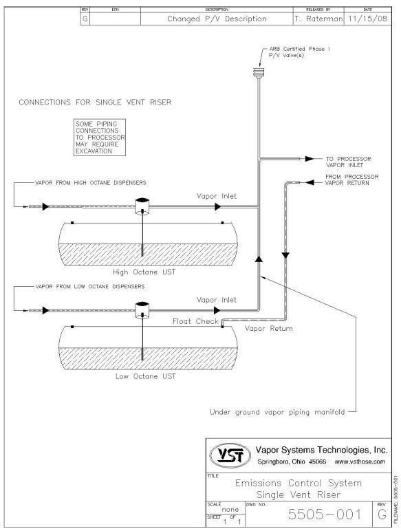
Figure 13: Processor Connections with Single Vent Riser
