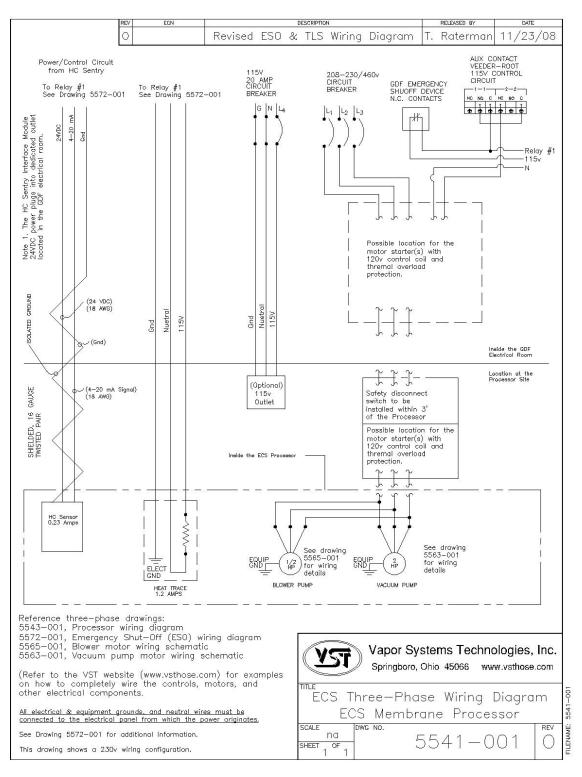
Figure 24: Processor Three-Phase Wiring Schematic
