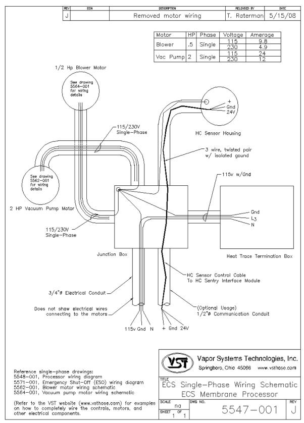
Figure 18: Single-Phase Wiring Schematic
