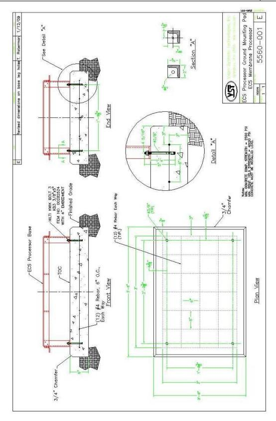
Figure 10: Processor Ground Mounting Pad
