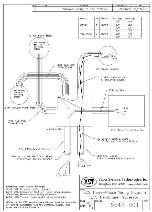
Figure 23: Processor Three-Phase Wiring Schematic
