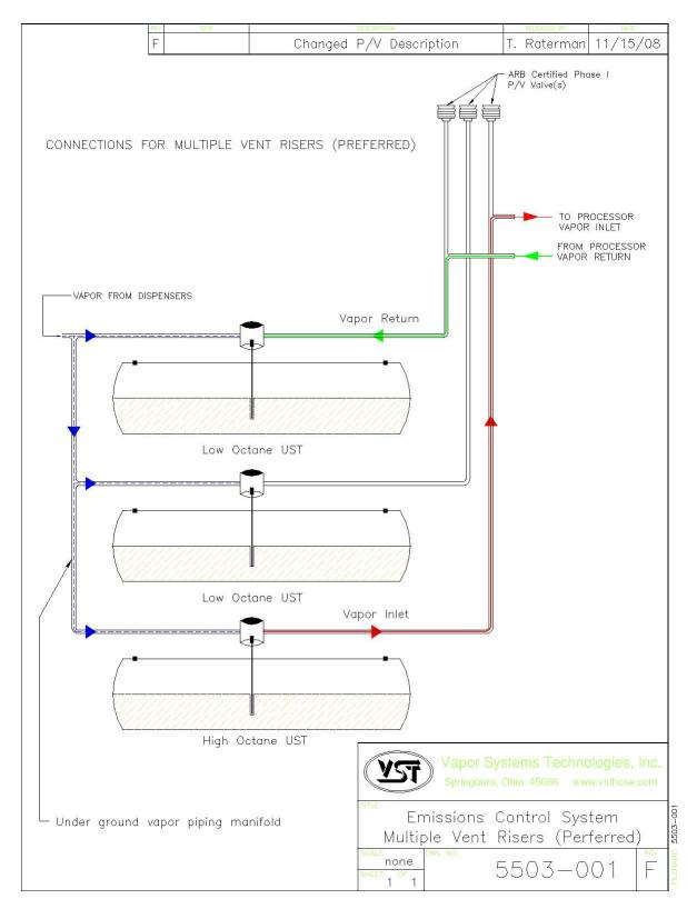
Figure 11: Processor Connections with Multiple Vent Risers
