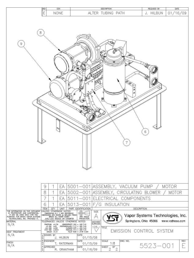
Figure 5: Processor Isometric Drawing (2 of 2)
