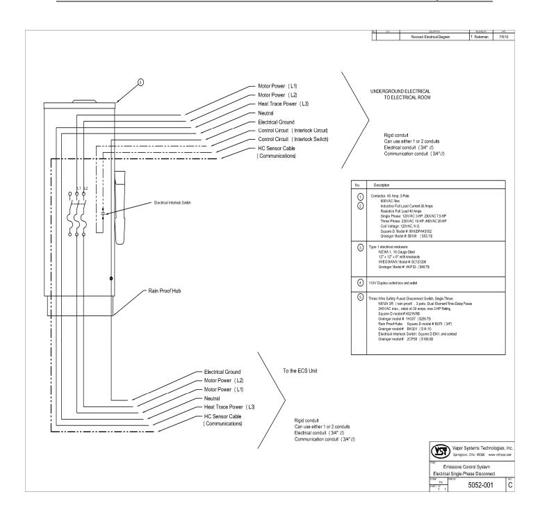
Figure 37: Single phase electrical disconnect
