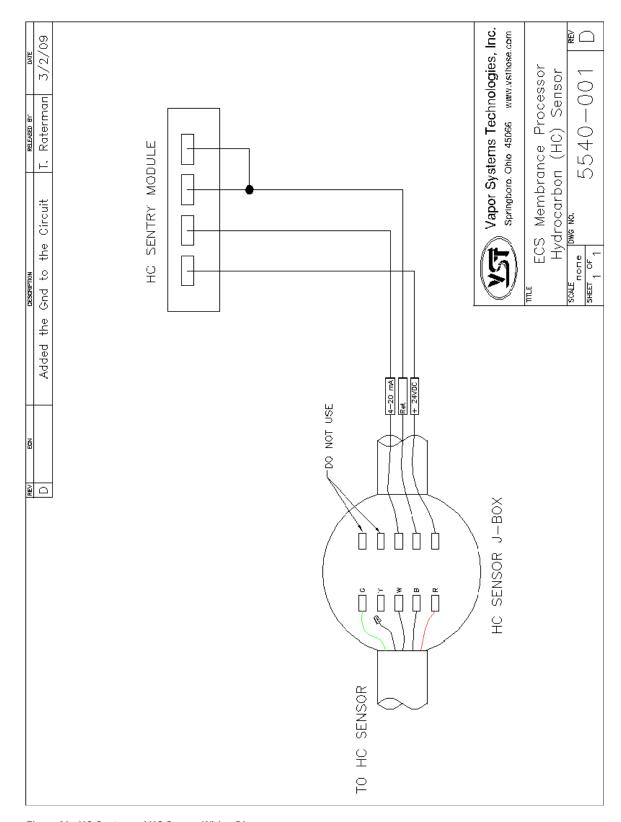
Figure 30: HC Sentry and HC Sensor Wiring Diagram
