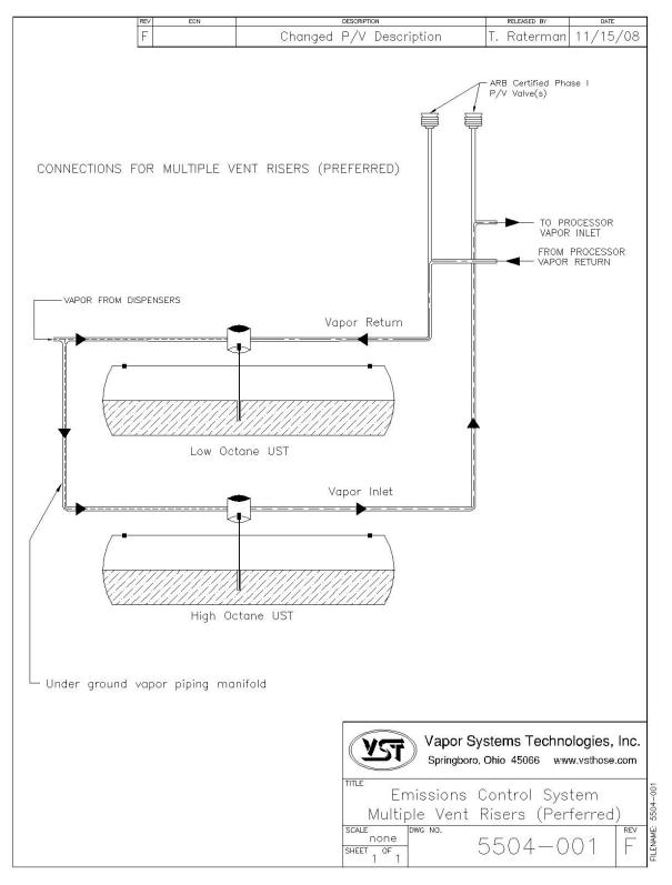
Figure 12: Processor Connections with 2 Vent Risers
