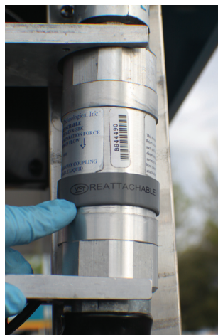
Figure 8: Reposition Retaining Sleeve
