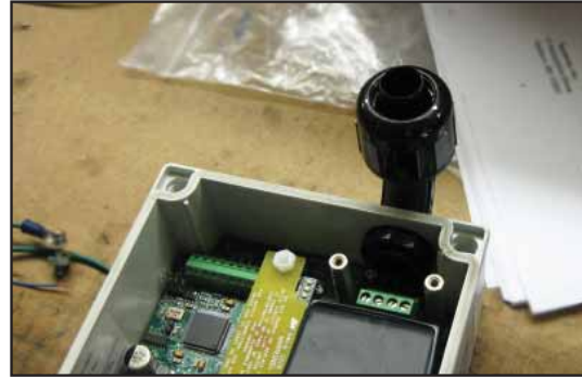
Figure 8: 90-Degree Fitting Installed
