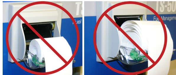
Figure 8: Do NOT load paper from door, Do NOT have paper wound loosely
