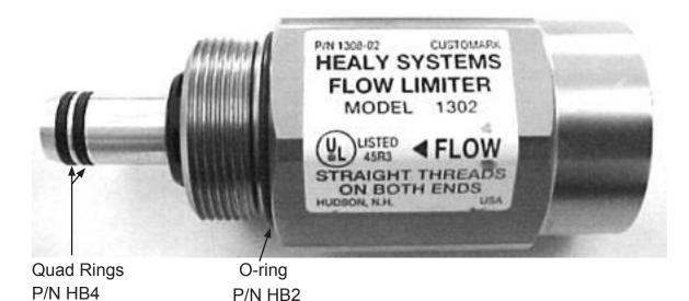
**The Healy Model 1302 Flow Limiter** is designed for installation into the female end of the Healy P/N 807 swivel breakaway before installation of a Healy Systems primary hose. The flow limiter reduces the product dispenser rate to conform to the U.S. EPA 10.0 gpm maximum dispensing limit.
