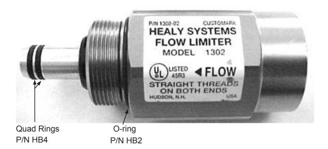
**The Healy Model 1302 Flow Limiter** is designed for installation into the female end of the Healy P/N 807 swivel breakaway before installation of a Healy Systems primary hose. The flow limiter reduces the product dispenser rate to conform to the U.S. EPA 10.0 gpm maximum dispensing limit.
